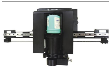
Auto Supply and Inspect Solder Paste
